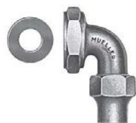
Quarter bend coupling Female extra strong (XS) lead flange thread x copper flare nut (pre-1920)
